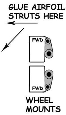
**GLUE AIRFOIL STRUTS INTO ENDS**
